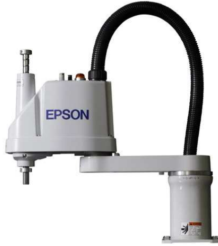
Figure 7.1: An EPSON Scara LS3: standard version.
