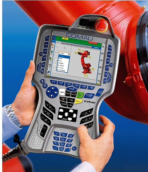
Figure 2.2: This Comau teach pendant is used to program various models of the robotic industrial machinery the company makes.
