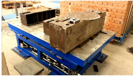
Figure 8.8: Physical shaking table in our laboratory.
