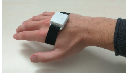
Figure 2.8 – The device is mounted on the back of the hand by means of an elastic strap.
