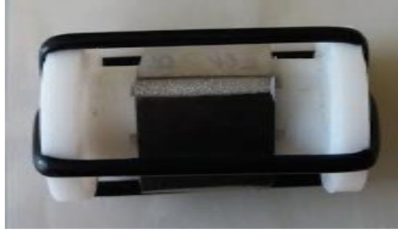
Figure 4-2: Customized Anderson device on the LPBF cubic specimens
