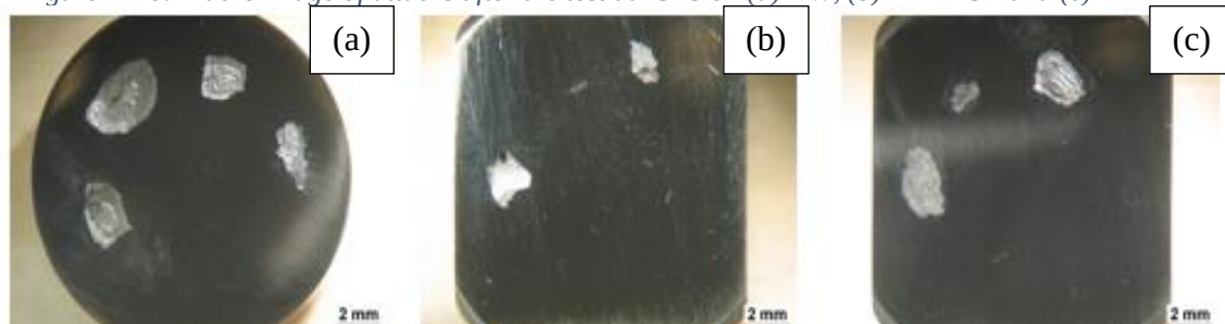
Figure A-11: Macro image of attacks after the test at 30°C on (a) HW, (b) LPBF UT and (c) LPBF HT
