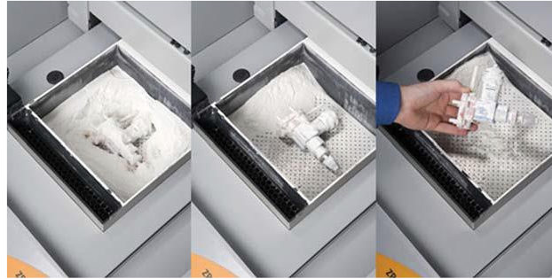
Figure 2-9: Automated powder removal using vibratory and vacuum assist in a ZCorp 450 machine 26
