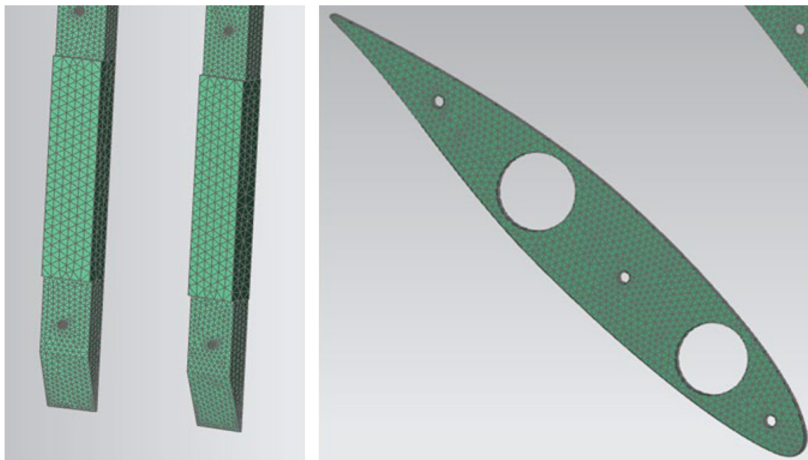
Fig. 10 Side cover (right figure), and support PVC insert (left figure),-strip 3D mesh
