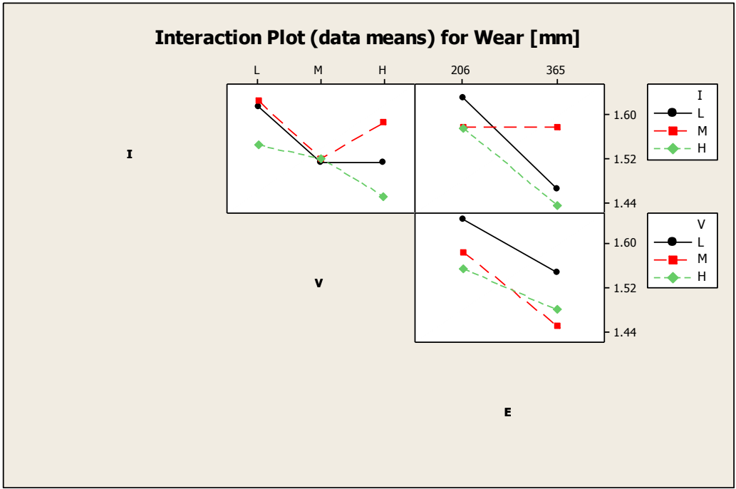
Figure 70: Interaction plot for electrode wear mean data as a function of I, V and E, d 150 \mu m
