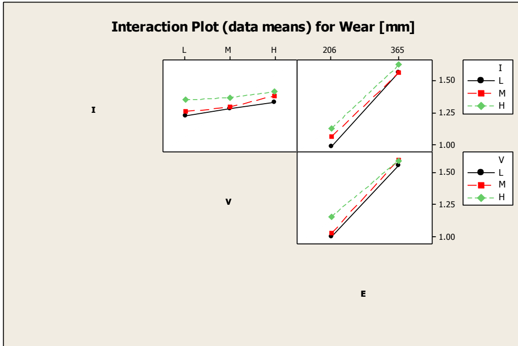
Figure 102: Interaction plot for electrode wear mean data as a function of I, V and E, d 300 \mu\text{m}
