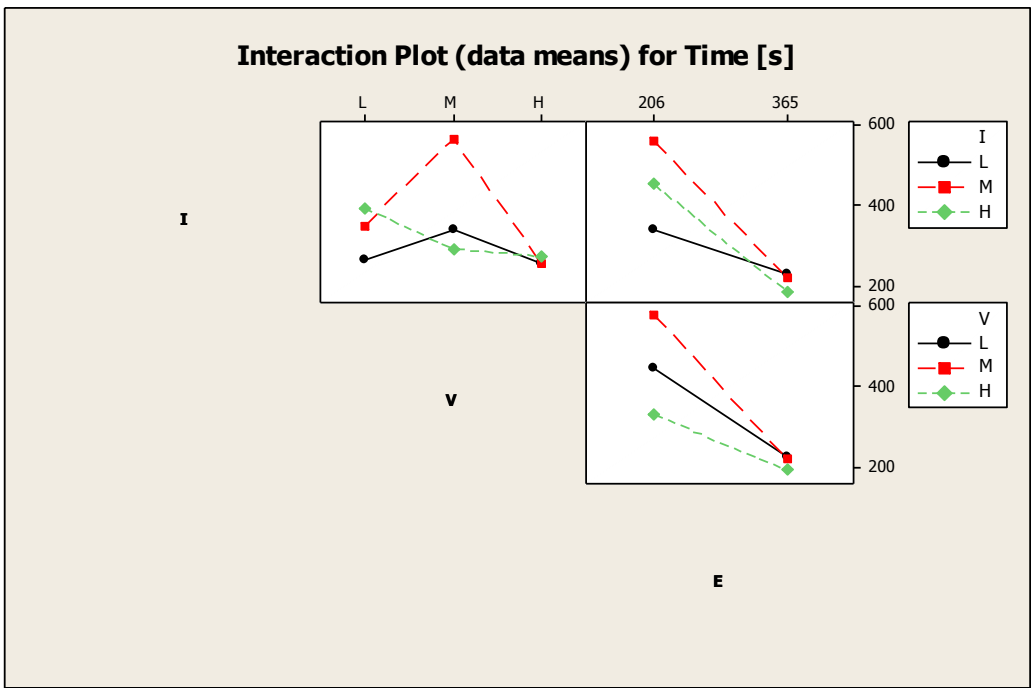
Figure 71: Interaction plot for machining time mean data as a function of I, V and E, d 150 \mu m
