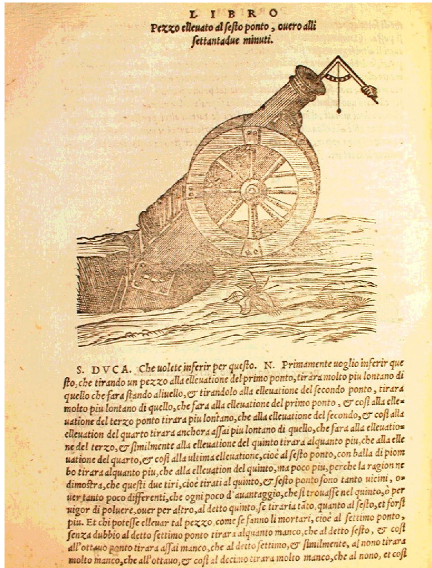
Fig. 1.17 Plate from Quesiti on inclined cannon for the maximum path and bombardier's quadrant 71
