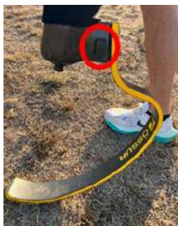
Figure 1: Set-up of Axivity AX6 sensor on a prosthesis socket
