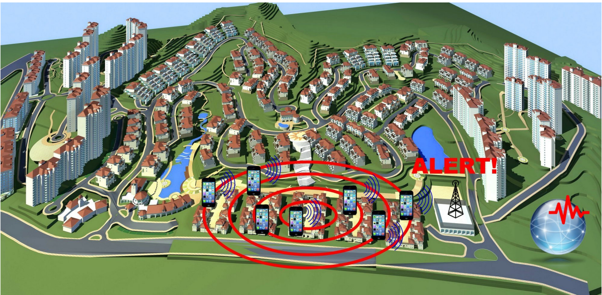
Figure 3.2: Visual representation of EQN. It uses the accelerometer in smartphones to recognize the shaking brought on by an earthquake in real time and sent an alert to user not too close to the epicenter. The image is taken from the website of the earthquake network project ( https://sismo.app/ ).
