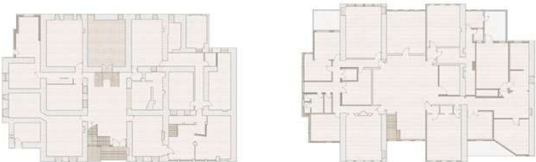
Figure 2. Ground and first floor plans of Libohova Villa
