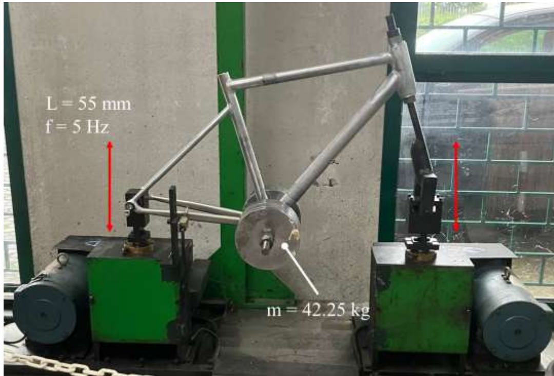
Figure 93 - Fatigue test rig used for frame testing, showing the imposed vertical stroke, loading frequency and total mass applied at the bottom bracket.
