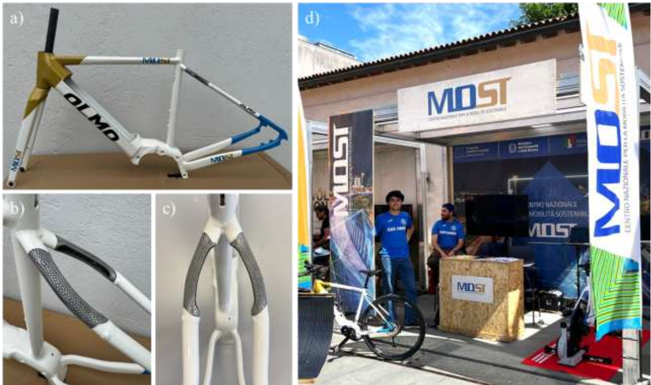
Figure 79 - (a) Prototype frame with the lattice structure component integrated into the rear triangle, (b,c) close-up views of the AlSi10Mg insert and (d) presentation of the prototypes during the Giro-E 2024 event.
