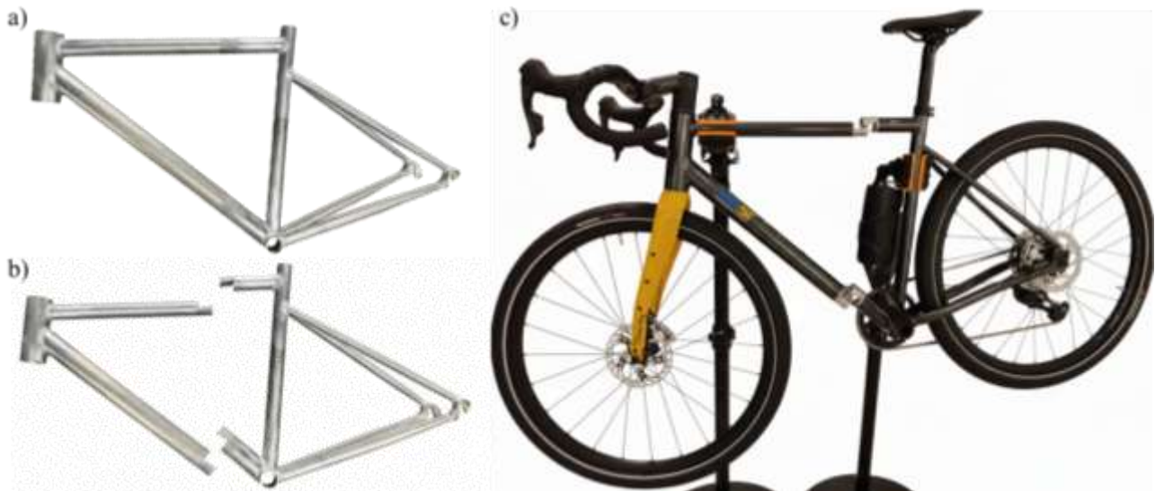
Figure 92 - Frame equipped with the joint prototypes in (a) assembled and (b) disassembled configuration; (c) complete bicycle prototype with electric motor and integrated joints.
