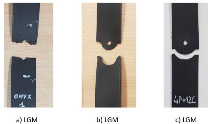
Figure 9. Failure modes in fibre concentric fill pattern: (a) LGM in Full Onyx samples, (b) LGM in 6C samples and (c) LGM in 12C samples.
