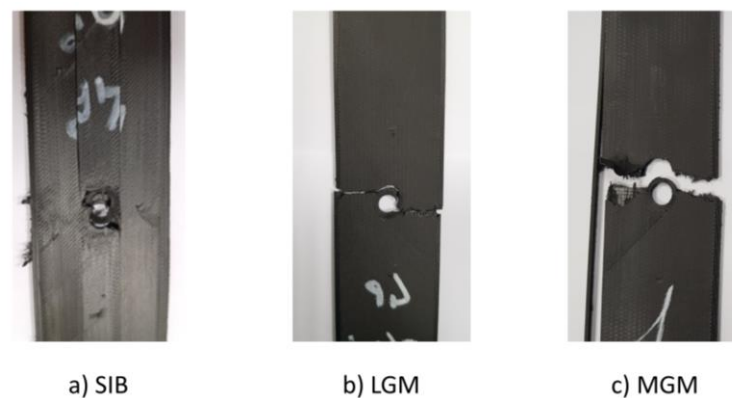
Figure 12. Failure modes in isotropic samples: (a) SIB in 0^\circ samples, (b) LGM in 0/90 samples, and (c) MGM in 0/90/45 samples.
