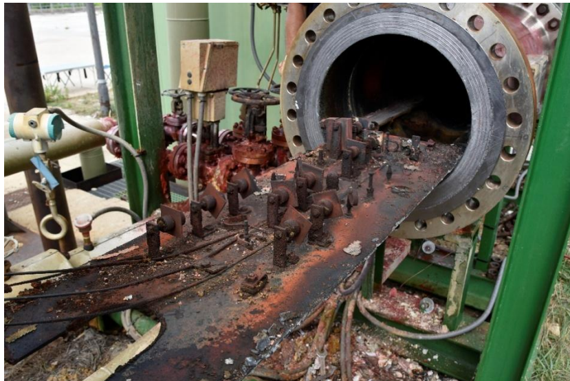
Figure 39 - Specimen plate with mounted samples after the field exposure test
