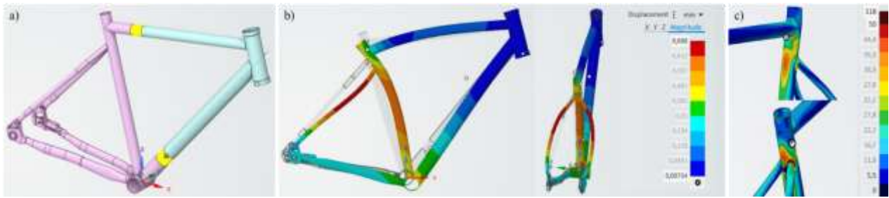
Figure 86 - (a) As-is frame model with highlighted inserts at the cut sections; (b) displacement field of the as-is frame under load and (c) detail of regions with highest stress concentration.
