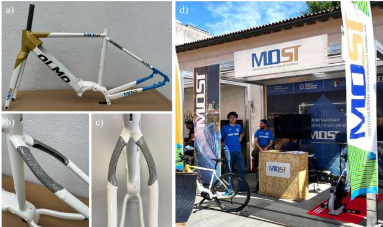
Figure 79 - (a) Prototype frame with the lattice structure component integrated into the rear triangle, (b,c) close-up views of the AlSi10Mg insert and (d) presentation of the prototypes during the Giro-E 2024 event.
