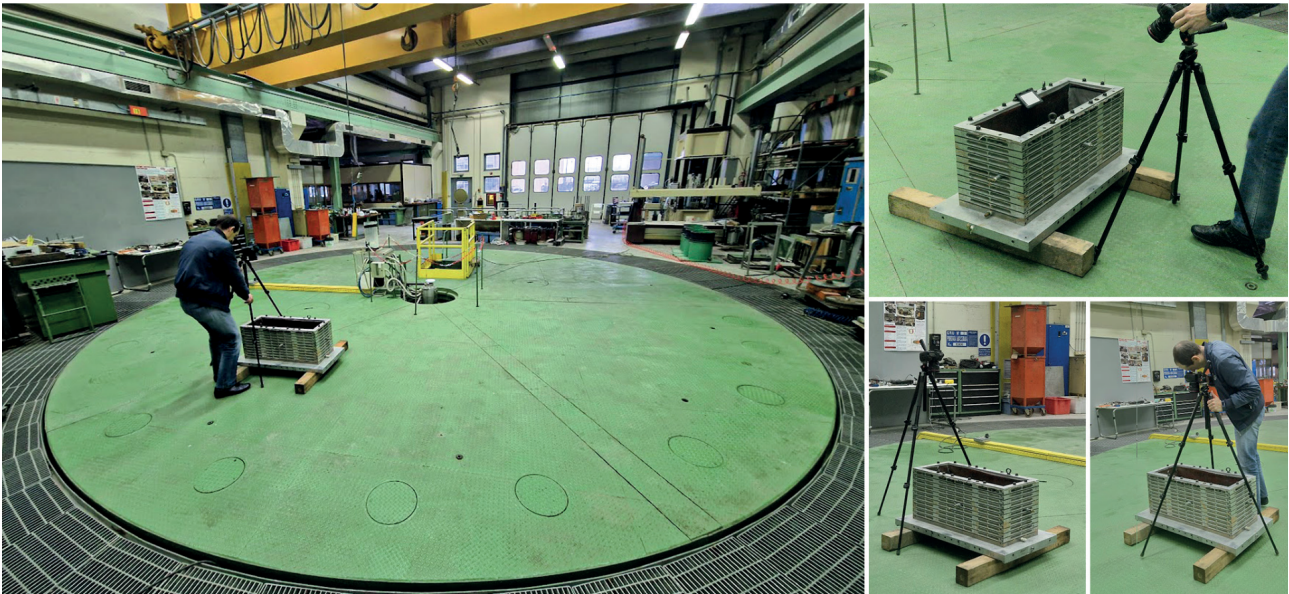
Figure 14: The photogrammetry data acquisition of the sample and the ESB support. Source: Cardaci, Giretti & Azzola (2024), CC BY 4.0.
