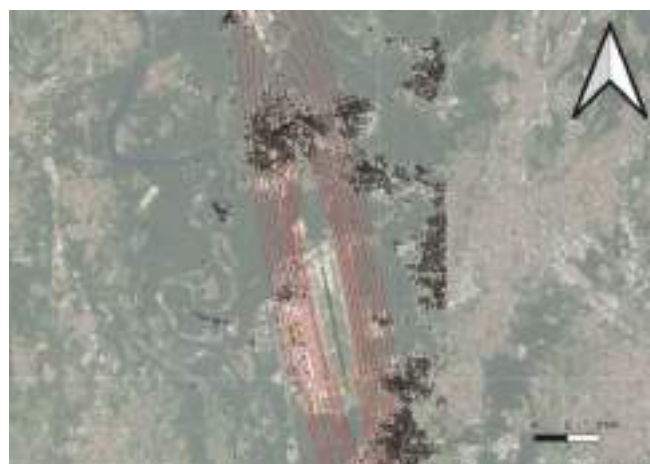
Fig. 12. Intersection of buildings data with noise contour NIZs for Milan Malpensa airport.
