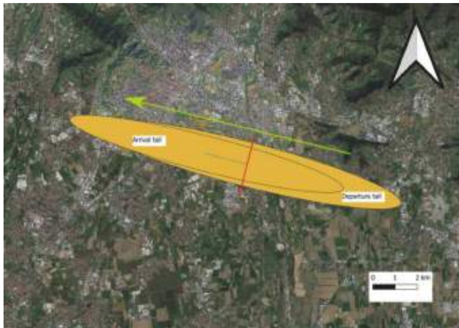
Fig. 14. An example of departure and arrival ellipses with their “tails” for a specific NIZ at BGY airport.
