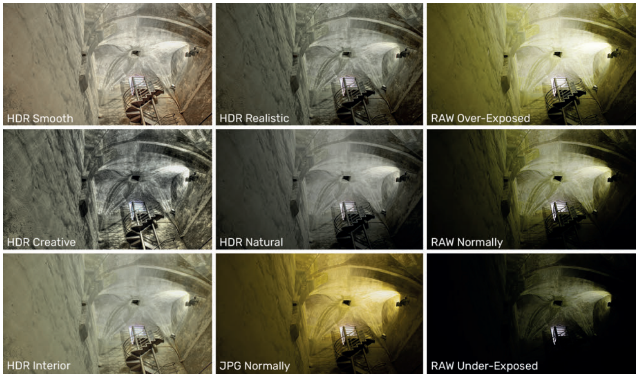
Figure 3. Photo processing: HDR images (8 bit tone mapping) and RAW images (12 bit).
