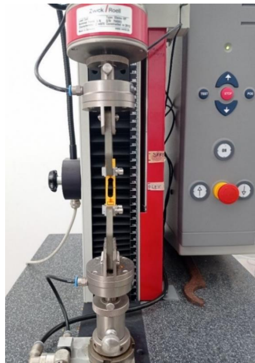
Figure 31: Zwick Roell 1 K dynamometer with a sample entered between the grips
