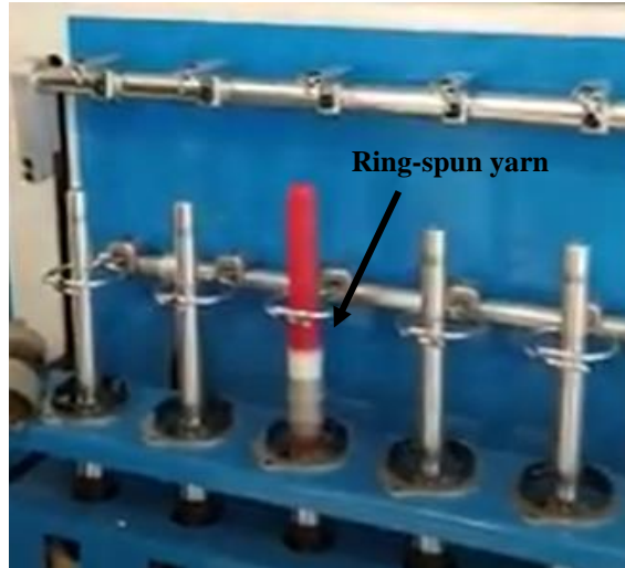
Figure 29: Ring spinning machine adopted with ring bobbin production
