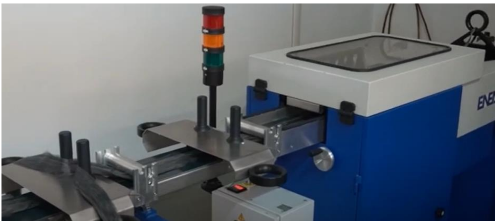
Figure 26: Drawing phase of the innovative spinning process
