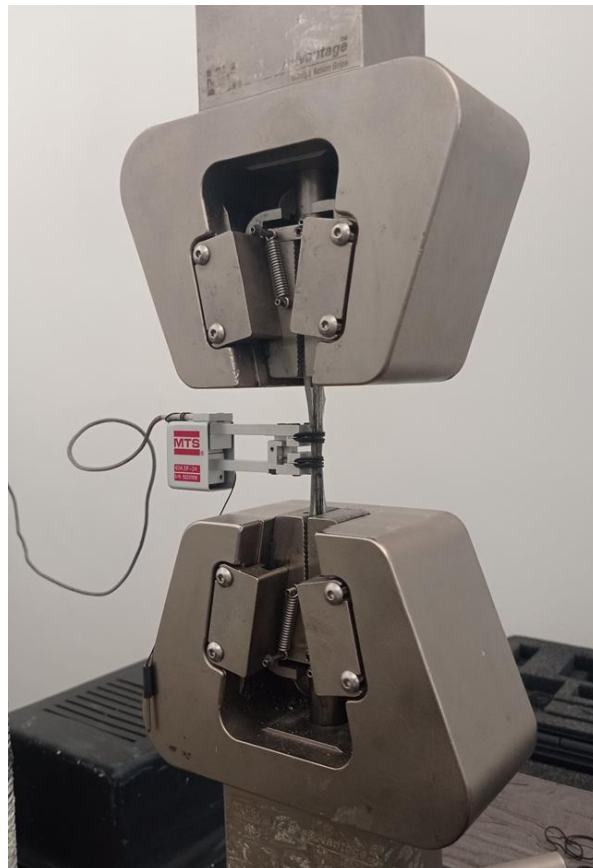
Figure 58: Self-tensioning grips and MTS ® contact extensometer used
