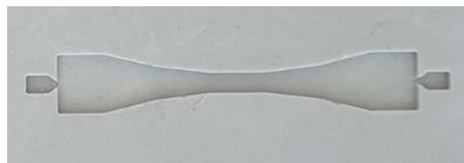
Figure 53: Geometry of the test specimens used
