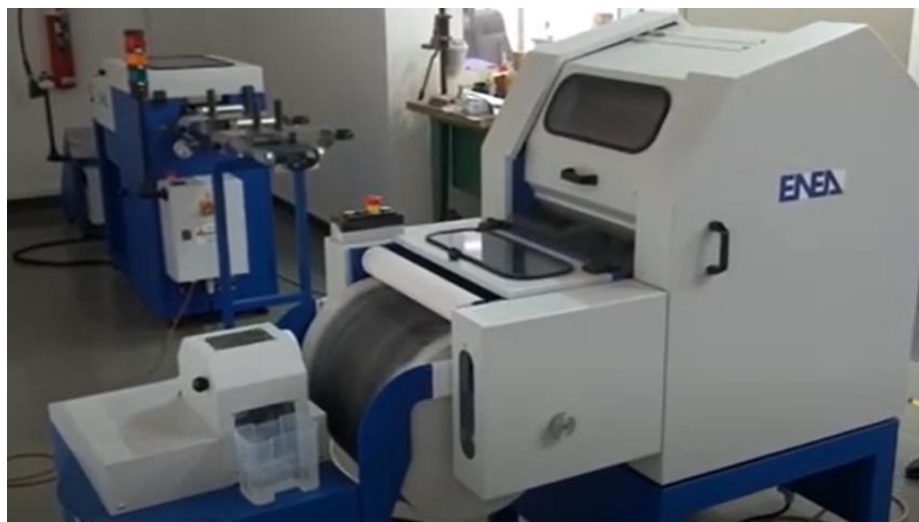
Figure 25: Carding phase of the innovative spinning process
