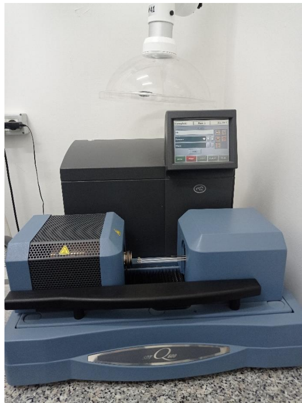
Figure 36: TA instruments SDT Q600 used for TGA and DSC
