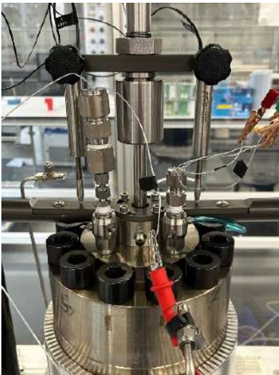
(c) Detail of the electrical connection for DCPD measurements in the autoclave.
