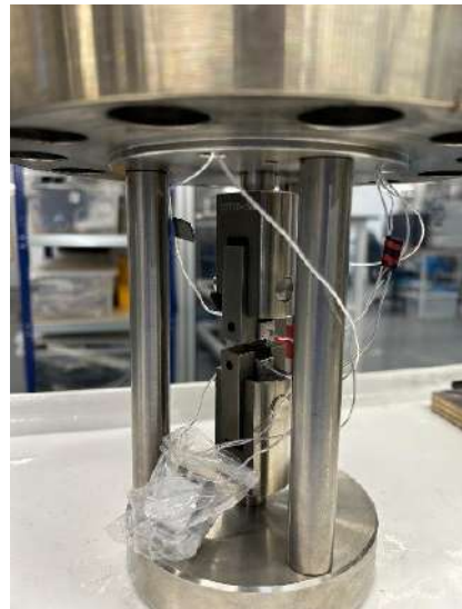
(d) Part to be inserted into the autoclave body, showing properly tested samples and a reference sample.
