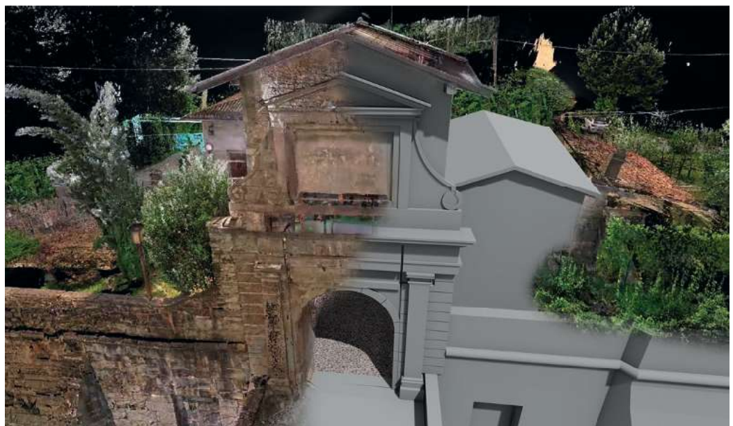
Fig. 9a. 3D survey and Scan-to-BIM model of Porta di San Lorenzo: comparison between acquired data, interpreted form and parametric reconstruction (S.A.B.E. 2025).
