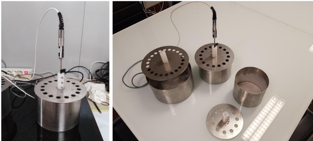
Figure 9. Test bench: (left) assembled system with pot, lid, and thermocouple; (right) different pot sizes (150, 180, and 210 mm).
