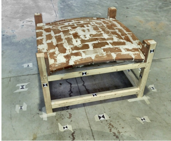
Fig. 3. Lowered vault built by T0, using the scaffold.
