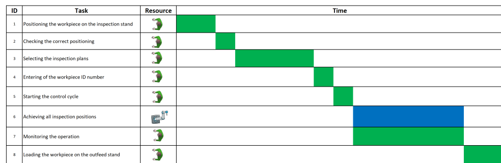
Figure 8. Task assignment related to the quality check of welding points performed in a collaborative manner.
