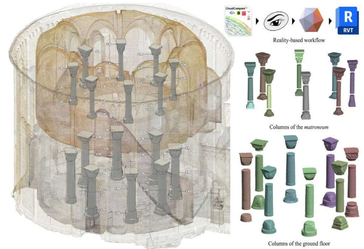
Fig. 5 - Semantic segmentation of the column elements encoded according to Rota Nodari [27]. From the left, superimposition between HBIM models and points cloud. On the right, reality-based segmented models. (@E.C. Giovannini).
