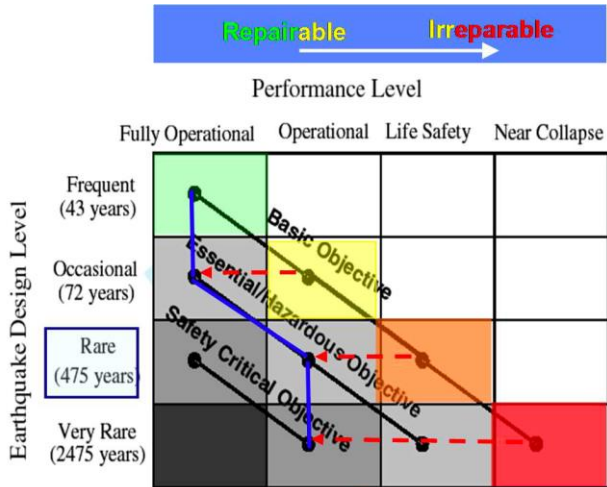
Figure V.3 - Rearrangement of the Seismic Performance Design Objective Matrix defined by the SEAOC Vision 2000 PBSE guidelines to match building tagging, and modification of the basic objective curve towards a damage-control approach (blue line). From [142].
