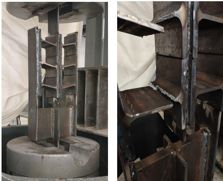
Figure VII.37 - Pictures of the test specimen of configuration III within the testing machine when failure is accomplished.
