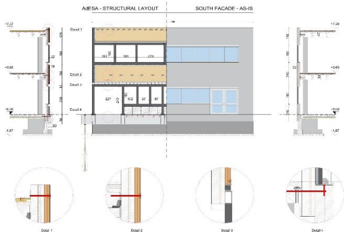
Figure VIII.22 - Representation of the structural intervention along the short facades of the building, showing some structural details: 1) steel dowels summit connectors between exoskeleton and pre-existence; 2) steel dowels intermediate diaphragm connectors; 3) detail of AdESA fuses; 4) structural connections of the new foundation. From [15].
