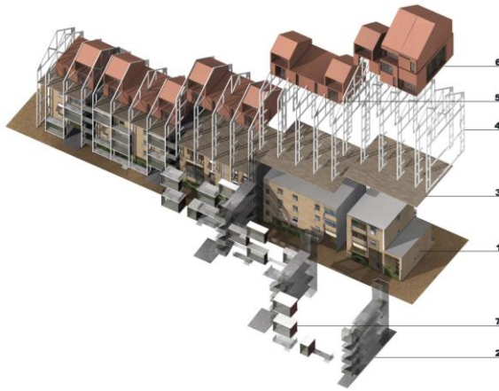
Figure IV.32 - Three-dimensional representation of the intervention concept: 1) existing building; 2) new staircase; 3) new slab above the existing building; 4) structural steel frames; 5) new timber apartments; 6) new common spaces and services; 7) "Small boxes" of volume extension in the façade. From [136].
