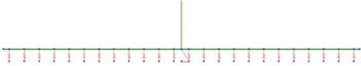
Figure 0.4 - FEM modelling to simulate the rocking and sliding shear behaviour at the base of precast panels using general-links.
