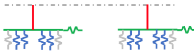
Figure VI.48 - Schematic representation of vertical general links at the base of CLT panels for configurations C and D. The end elements representing the sacrificial fuse toes are highlighted in grey.
