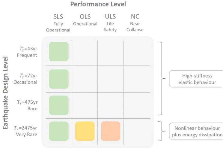
Figure VI.8 - Matrix of the seismic performance design objectives for adaptive exoskeletons, indicating conceptual structural behaviour for each earthquake design level.
