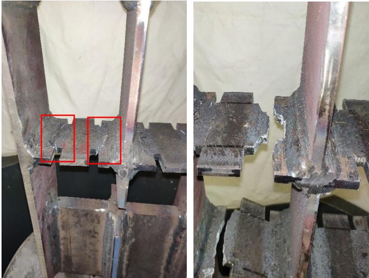
Figure VII.35 - On the left-side: Image of crack propagation from the corners of the slits. On the right-side: Image of the fracture of the reduced section at the end of the test.
