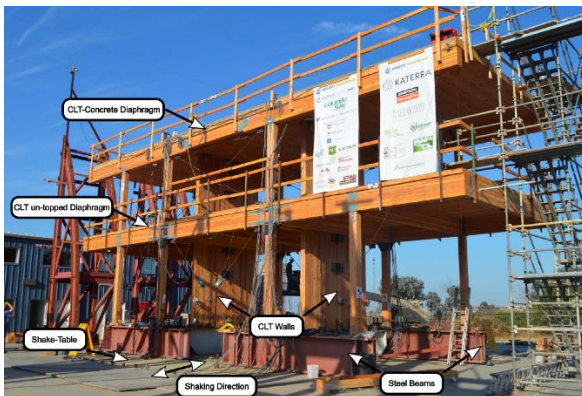
Figure VI.6 - Image of the two-story CLT prototype structure being tested on a shaking table at the USDC during the summer of 2017. From [160].
