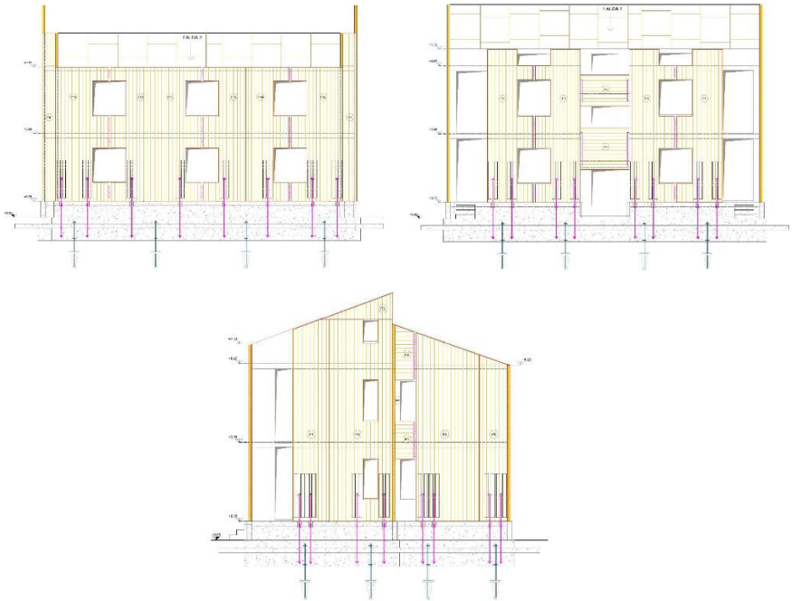
Figure IX.12 - Representations of the timber exoskeletons arranged along the main façades, in which the wooden elements are shaded in yellow and the Dywidag bars in purple. From [248]
