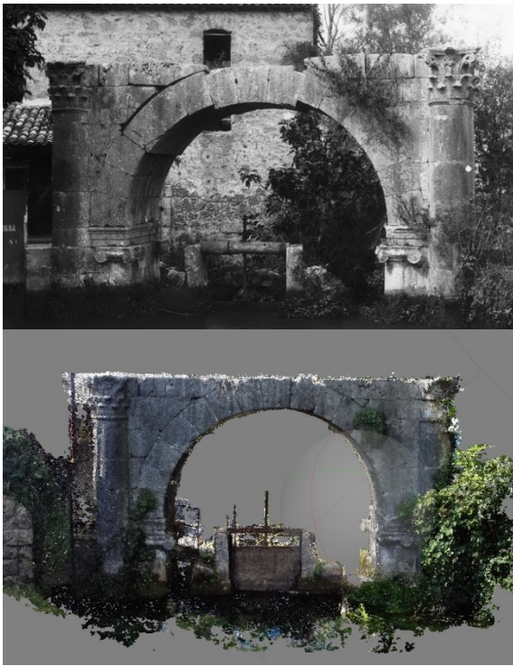
Figure 17. Arch of Marco Antonio: photograph taken in the early 1900s by the Germanic Archaeological Institute in Rome (a); 3D model from the elaboration with image-based technique of the photogrammetric survey data (b).
