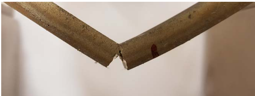
Figure 103: Bending failure in Functionally Graded Materials produced via DLD.
