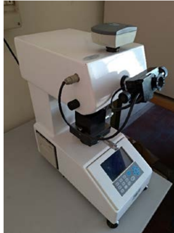
Figure 26: Vickers Microhardness instrument: Tecmet 2000.
