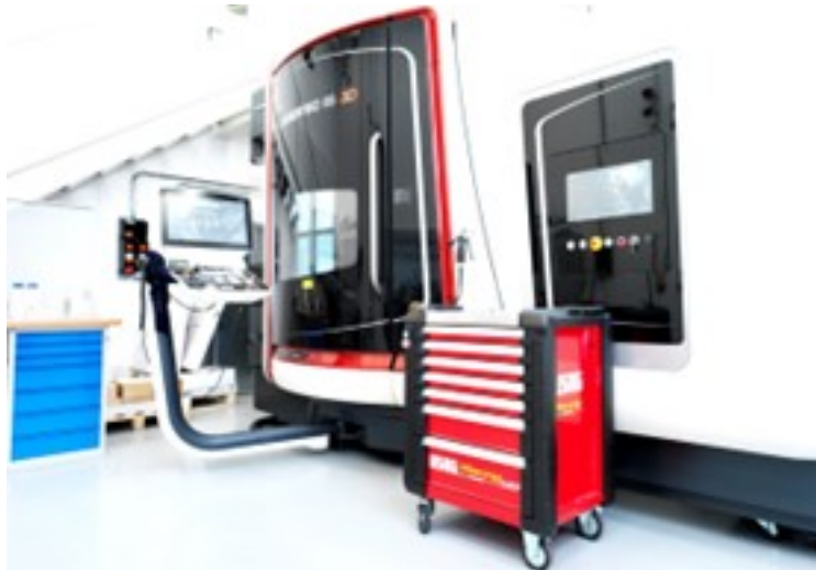
Figure 12: DMG MORI Lasertec 65 3D Hybrid machine used for all laser depositions.
