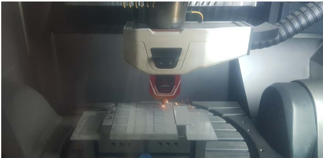
Figure 56: Deposition of the H13 single layers on 316L base-plate.
