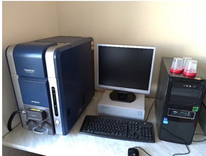
Figure 24: Hitachi TM3000 Tabletop SEM.
