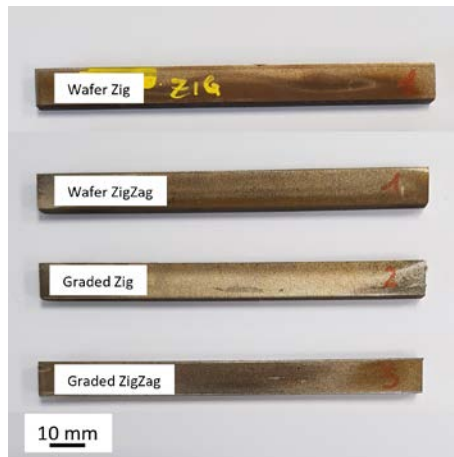
Figure 93: Graded and Wafer specimens, deposited with Zig and ZigZag strategies, for 3PB tests.
