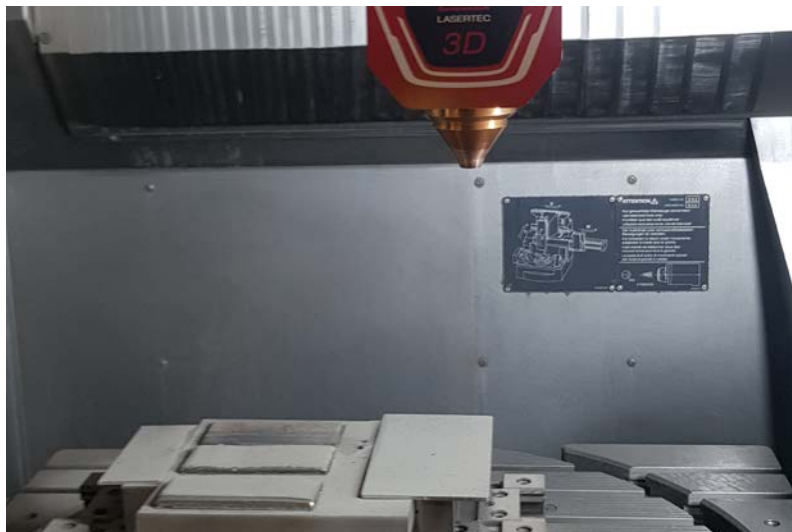
Figure 88: Direct Laser Deposition process of FGM structures in Lasertec 65.
