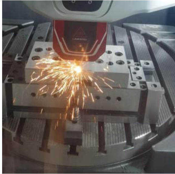
Figure 39: Laser head of Lasertec 65 during the first H13 single track deposition on 316L substrate.
