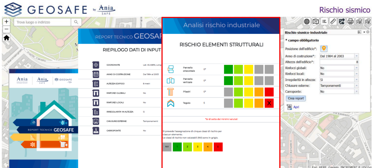
Fig. 14. Example of GEOSAFE output showing the component-based vulnerability matrix for a precast industrial building.
