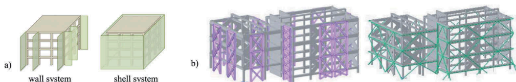
Figure 2. A) concept of structural exoskeletons conceived as wall or shell systems (adapted from Marini et al. 2017); b) application of steel wall and shell (diagrid) system to a reference case study (from Passoni et al. 2022b).
