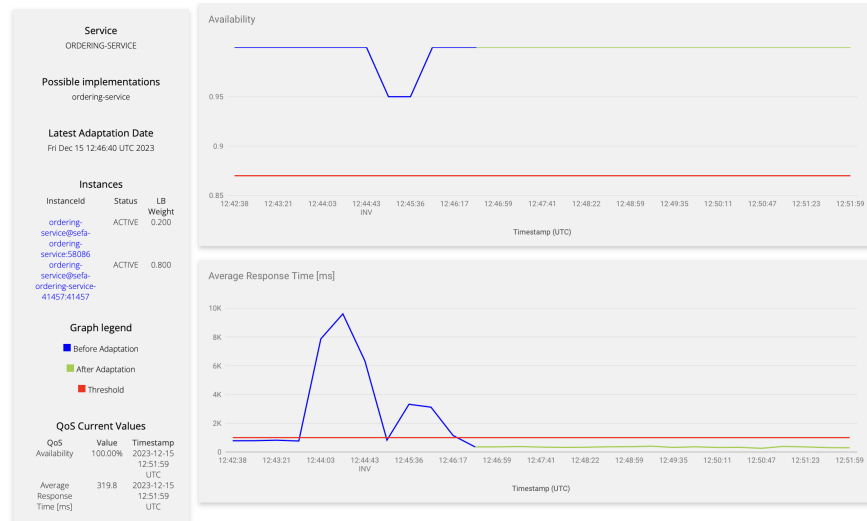
Figure 5: Screenshot of the dashboard showing QoS data of the managed microservices at runtime.
