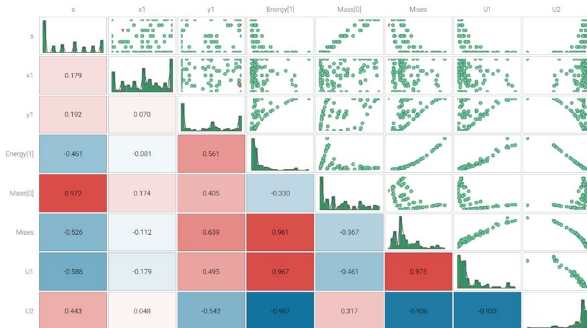
Figure 11. Scatter matrix—Abaqus—modeFRONTIER optimization analysis. The structure of this scatter matrix is the same as in Figures 4 and 8. Red markers are used in the histograms and scatter plots to indicate failed simulations.
