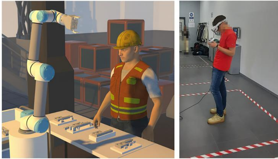
Fig. 2 VR environment for human–robot collaboration
