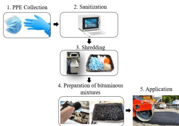
Fig. 1. Circular economy process steps: from waste PPEs to reinforced bituminous mixtures
