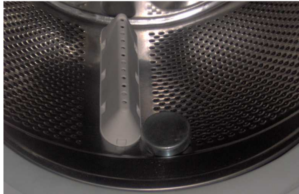
Fig.7. Magnet placed inside the drum, to emulate an unbalanced load.
