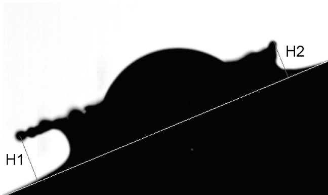
Figure 8 Sketch of splashing heights of leading edge ( H_1 ) and trailing edge ( H_2 ).
