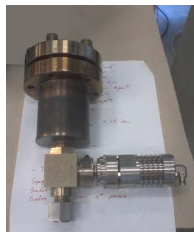
Figure 1: The injection system after its use. The heater had been removed and is not shown.
