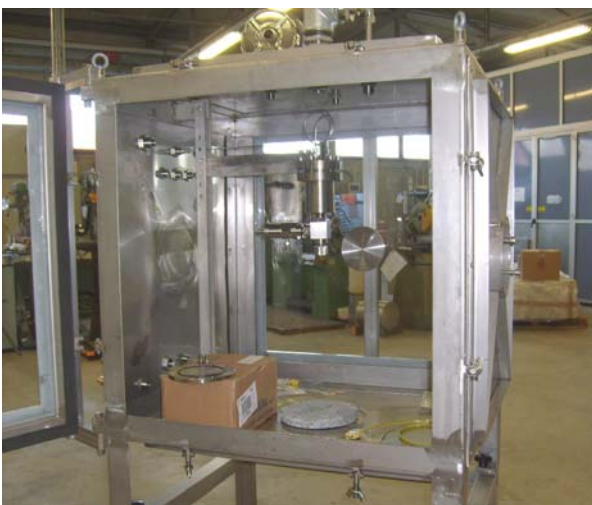
Figure 2: The test cell. The injection system is mounted to spray downward. The concrete target lays on the cell floor.
