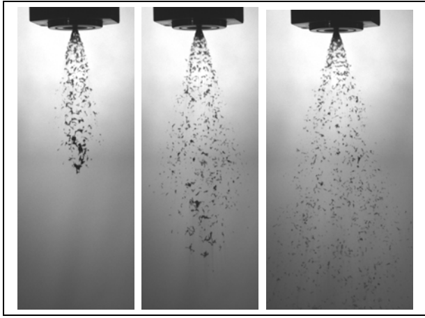
Figure 10: Images from Nozzle 0.40 mm, in air, sodium at 9 bar. initial spray development
