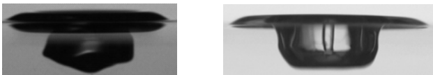
Figure 1: Differences in the experimentally obtained level of detail for the two test cases: crater evolution without (left) and with (right) wall effect for later stage of drop impact.
