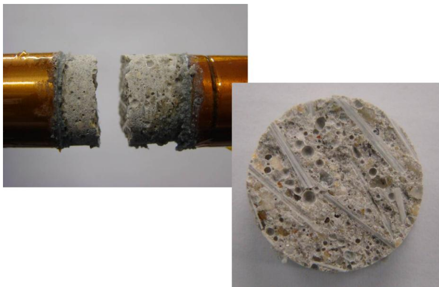
Figure 5 – Direct tensile strength test and perpendicular section of GF reinforced mortar.
