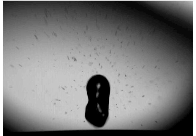
Figure 6: Typical outcome of drop impact on a surface at a temperature below the dynamic Leidenfrost point and low Weber numbers ( T = 250^{\circ}\text{C} , We = 40 ): the drop bounces and simultaneously scatters secondary droplets.
