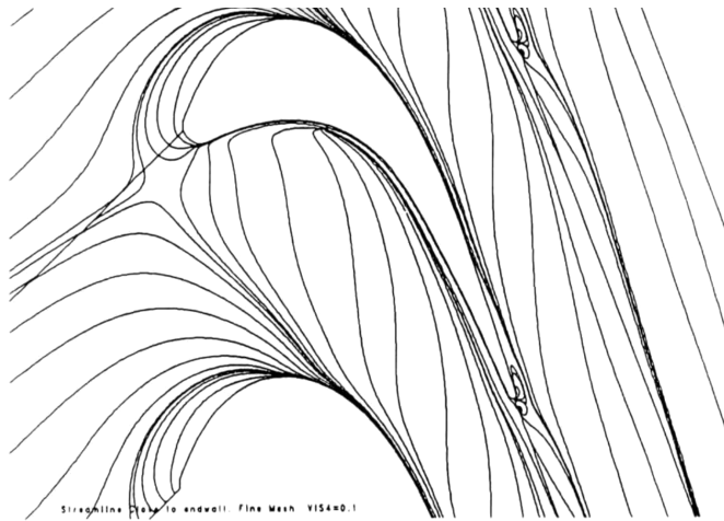
Figure 1.3: DLR cascade geometry and computed endwall streamlines - [22]
