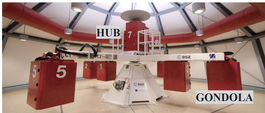
Fig. 6: Large Diameter Centrifuge: hub and gondolas.
