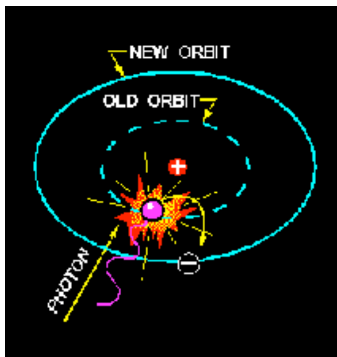
Image 60: illustration of a photon leap. Every electron has a specific orbit around an atom. This orbit relates to the level of energy it possesses. A passing photon can impart energy to the orbiting and push it into a higher energy orbit. Image source: www.tpub.com/neets/book1/chapter1/1c.htm
