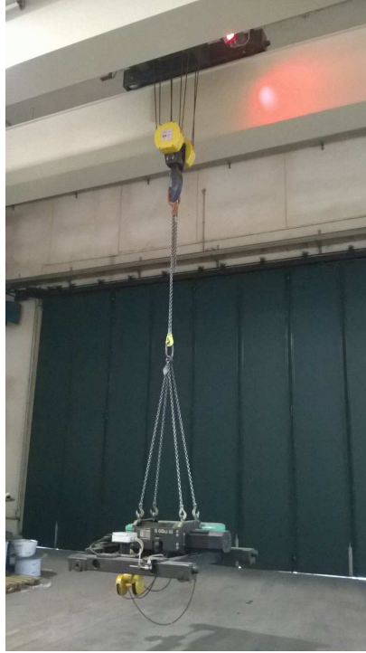
Figure 3.25: The triple pendulum case on the real bridge crane.
