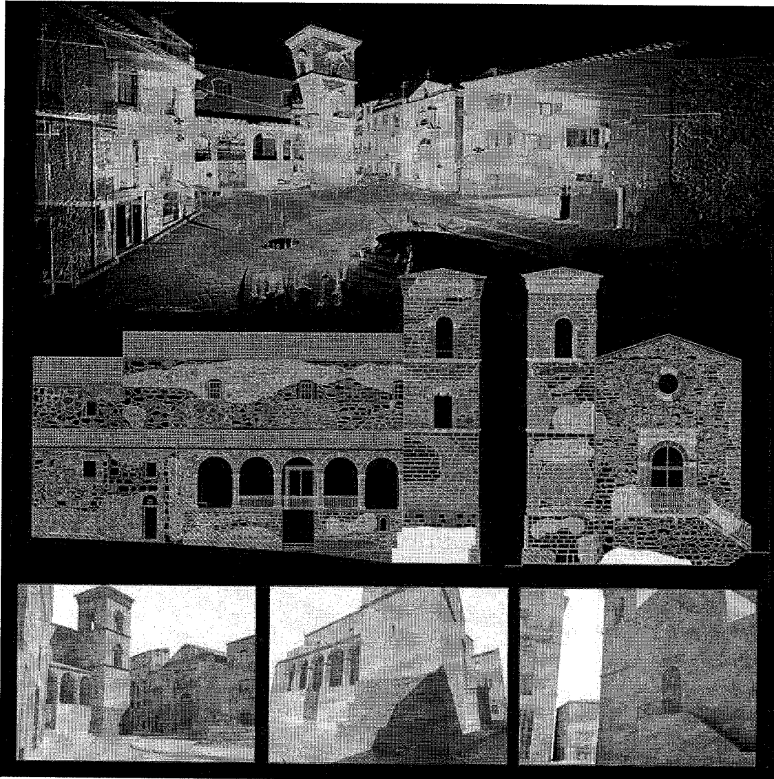
Figure 3. The Church of St. Tommaso (3D Scanner Model, 3D Cad Model and traditional draw).
