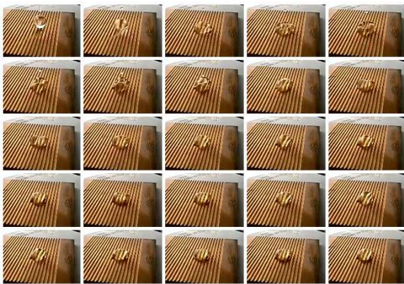
Figure 16: Drop deposition on the brass 400 \mu\text{m} microfin surface: experimental video acquisitions at 240 fps.
