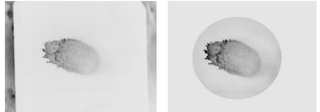
Figure 9: Wall film raw image (left), Wall film image energy and profile corrected (right)
