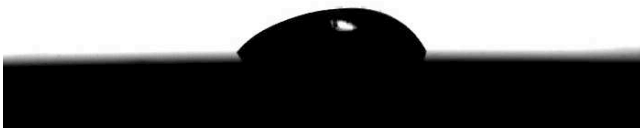
Figure 2: Typical outcome of drop impact on a surface at a temperature below the boiling point of the liquid ( T = 100^\circ\text{C} , We = 100 ): the drop is deposited on the surface and convection is the main heat transfer mode.
