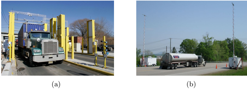
Figure 2.9: Standard radiation portal monitor (a) used to scan commercial traffic for radiation sources and advanced concept of portal monitor based on video tracking and gamma-ray imaging (b).
