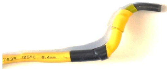
Figure 2.12: Completed single Ti-MMO probe.
