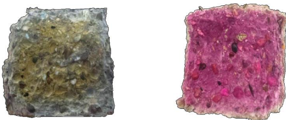
Figure 3.31: Visual analysis of "EXP3" concrete surface after spraying with modified Indigo Carmine (left) and phenolphthalein (right) pH indicators, at 28 days of ageing.
