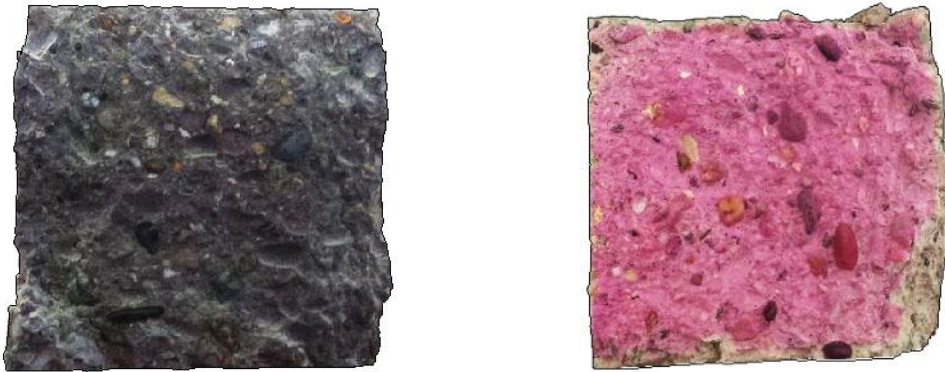
Figure 3.30: Visual analysis of "EXP2" concrete surface after spraying with modified Indigo Carmine (left) and phenolphthalein (right) pH indicators, at 28 days of ageing.
