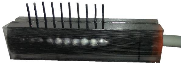
Figure 2.10: Completed MEP probe.
