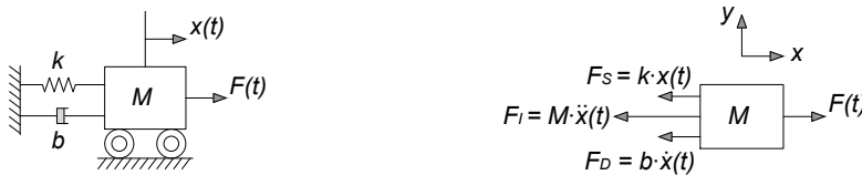
Figure 3.17 Single degree of freedom scheme adopted for the structure (to the left) and the free body diagram of the structure model (on the right).
