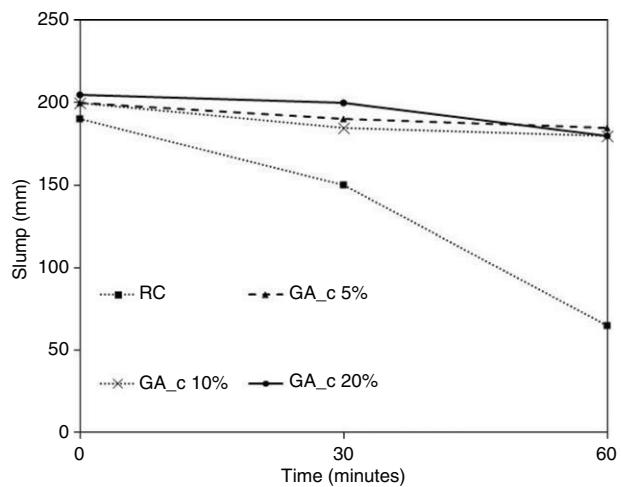
FIGURE 6. Slump loss of GA concretes ( $w/c=0.45$  and  $350 \text{ kg}/\text{m}^3$  cement content) and reference concrete ( $w/c=0.53$  and  $330 \text{ kg}/\text{m}^3$  cement content).
