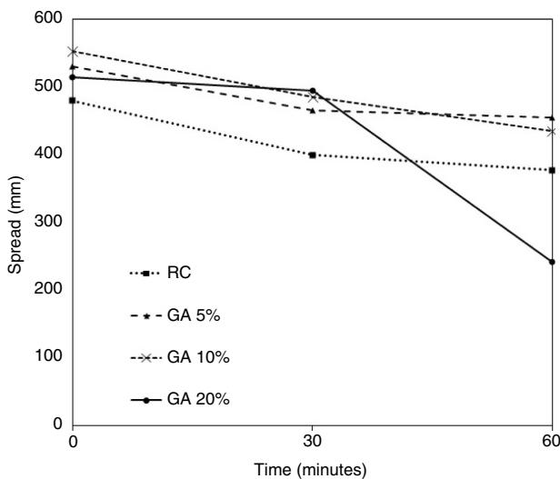
FIGURE 4. Flow value of GA and reference concretes as a function of time with  $w/c=0.53$  and  $330 \text{ kg}/\text{m}^3$  cement content.
