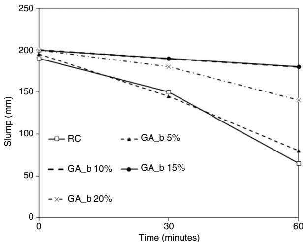
FIGURE 5. Slump loss of GA concretes ( $w/c=0.45$ ) and reference concrete ( $w/c=0.53$ ) at  $330 \text{ kg}/\text{m}^3$  cement content.
