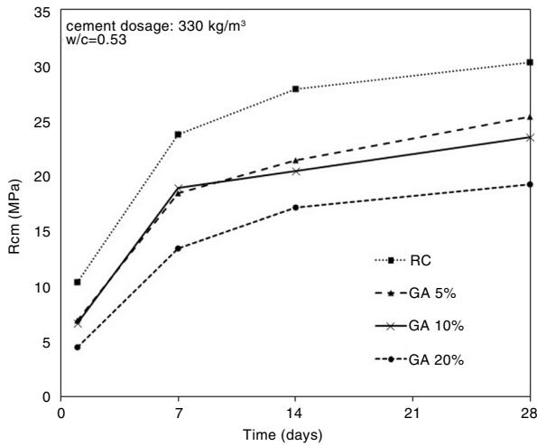
FIGURE 7. Compressive strength vs. age of GA and reference concretes with  $w/c=0.53$  and  $330 \text{ kg}/\text{m}^3$  cement content.
