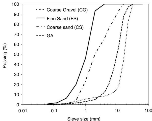
FIGURE 1. Grading of natural and GA aggregates.
