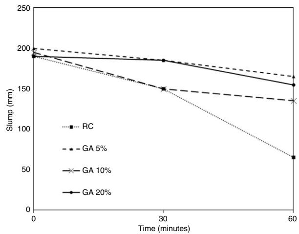
FIGURE 3. Slump loss of GA and reference concretes with w/c=0.53 and 330 kg/m<sup>3</sup> cement content.
