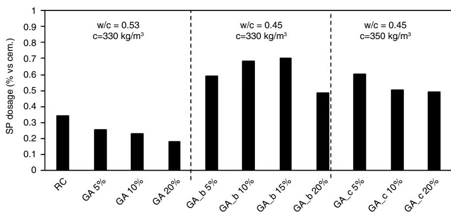
FIGURE 2. SP dosage for all concrete mixtures.
