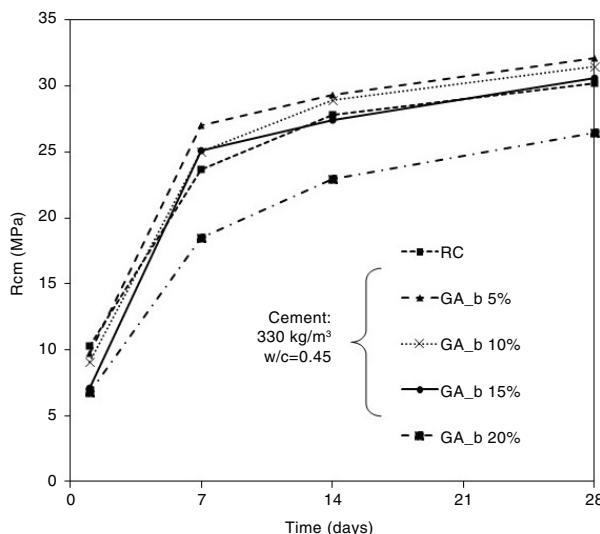
FIGURE 8. Compressive strength vs. age of GA concretes (w/c=0.45 and 330 kg/m<sup>3</sup> cement content) and reference mixture (w/c=0.53 and 330 kg/m<sup>3</sup> cement content).
