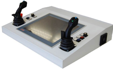
Fig. 8. Control panel of the Remote Manipulator Control
