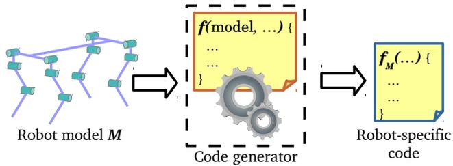
Fig. 6. Generation of an implementation of dynamics algorithms tailored for specific robots. The code generator must embed the knowledge about the abstract algorithm. A concrete implementation is achieved by turning the algorithm into code in some language, where the references to the robot model are substituted with actual values and specific instructions.
