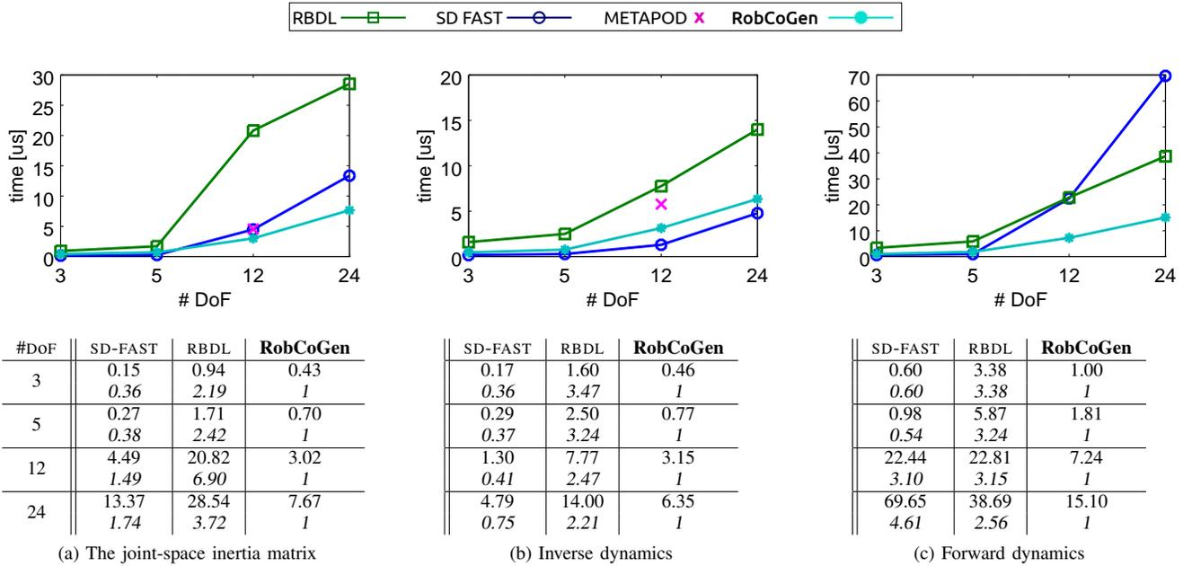
Fig. 12. Performance comparisons between the C++ code generated by RobCoGen and RBDL, SD-FAST, Metapod– for three dynamics routines. The plots at the top show the absolute, average execution time in  $\mu s$  versus the number of degrees of freedom of the robot model. The tables at the bottom refer to the same results, and show the absolute execution time (regular font) as well as the ratio with the execution time of RobCoGen (*italic font*).
