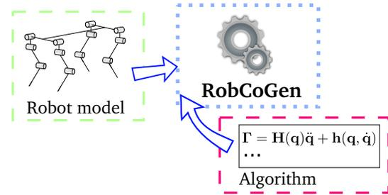
Fig. 15. Ideal inputs of RobCoGen. Having an independent model of the algorithm, in addition to the model of the robot, would make the code generator more extensible.
