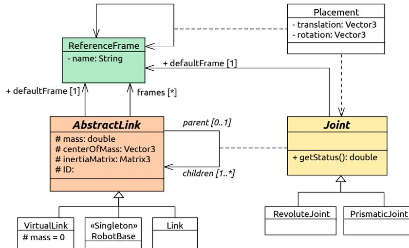
Fig. 3. The kinematic tree meta-model as an UML class diagram. It can represent multibody systems, capturing the role of a joint as the connection between a parent-child pair of links, and emphasizing their association with reference frames. The convention about the placement of these frames (that cannot be modeled in the diagram) and the parameters about the relative pose of two successive ones (the `Placement` class) provide the full geometry information about the robot.
