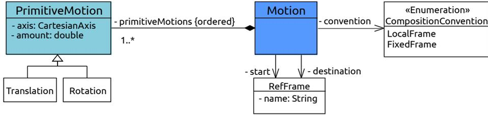
Fig. 2. A UML class diagram representing rigid motions. A `Motion` is a sequence of movements, rotations and translations, a generic body has to perform to go from one pose to another pose; poses are represented by reference frames. The interpretation of the ordered sequence of primitive motions is unique because of the `CompositionConvention` property.
