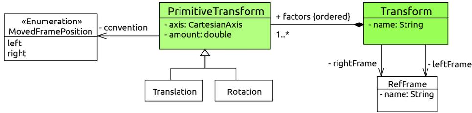
Fig. 1. The UML class diagram for coordinate transforms. A generic, named `Transform` results from the product of several `PrimitiveTransform`s, which correspond to pure rotations or translations. The `MovedFramePosition` property allows to determine uniquely any primitive transform.
