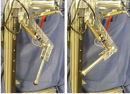
Fig. 13. The hydraulic leg of the HyQ robot.
