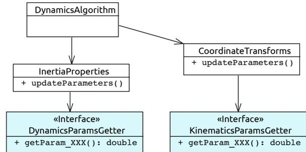
Fig. 10. Simplified layout of the C++ classes dealing with dynamically changing parameters, as generated by RobCoGen (the Jacobians class is not shown). The illustrated dependencies enable the kinematics/dynamics to consistently reflect a change of the parameters. Changes only depends on the user implementation of the interfaces (in light blue).
