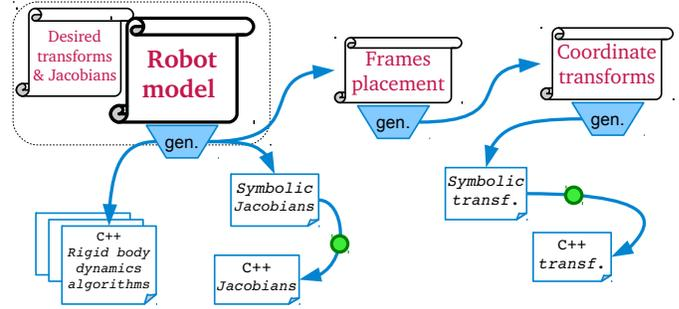
Fig. 8. Overview of the RobCoGen workflow. Scrolls represent DSLs documents (left to right: configuration DSL, Kinematics-DSL, Motion-DSL, Transforms-DSL); the trapezoids are code generators, while the sheets are generated source files. The green circle indicates a code generation step requiring the symbolic engine. The user only provides the robot model and a configuration file, as the other DSLs documents are also generated.
