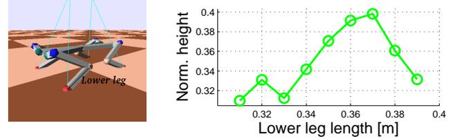
(a) Squat jump varying the length of the lower legs (the upper leg is 36.4cm long). The plot shows the distance traveled by the trunk, from the lift-off position to the apex of the jump, normalized by the lower leg length. The trunk is roughly  $90 \times 30$ cm long.
