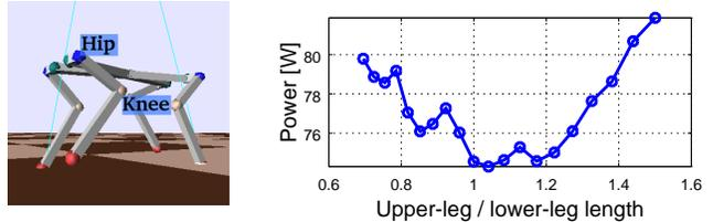
(b) Mechanical power employed by the hip and knee of one leg of the quadruped during trotting. Each data point is the average value over a single step. The  $x$  axis shows the ratio of the length of the upper and lower leg.
